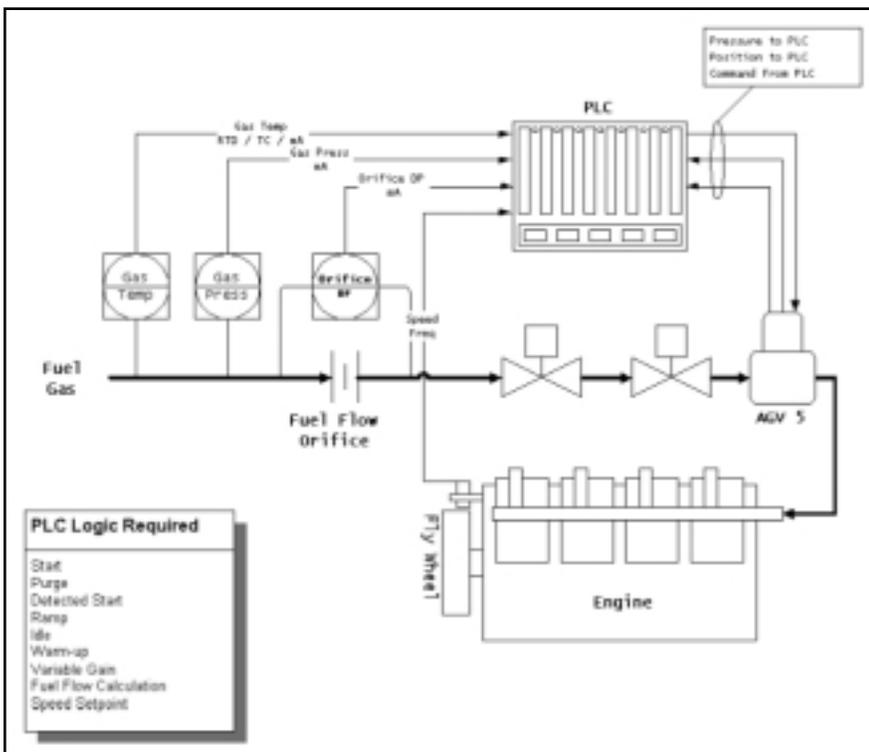
point in order to control the process gas flow without changing the pocket settings. The best fuel economy is achieved by operating the engine at its rated torque at all times and changing the engine speed to adjust the process flow. The governor must maintain speed within an acceptable tolerance with the ability to accept load changes with only a momentary speed transient.
