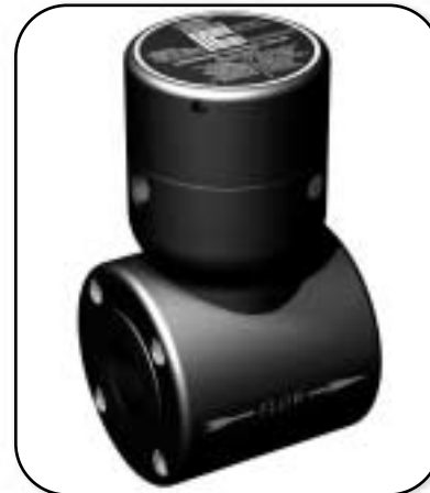
Continental Controls Corp. (CCC) has introduced an emissions control valve, the model ECV-5, that is designed to control the air-fuel mixture of natural gas-fueled, reciprocating engines. The ECV-5 and its O 2 sensor are designed for use with carbureted natural gas engines from 75 to 750 kW.
