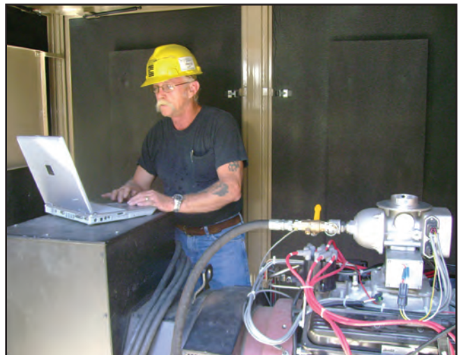
■ David Campbell of CCC sets up the EGC 2 on a GM 5.7 L gas engine.
