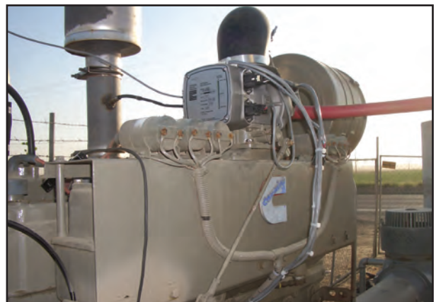
■ The EGC 4 is mounted on a Cummins G 855 Agricultural Pump in Tulare, California, U.S.A.
