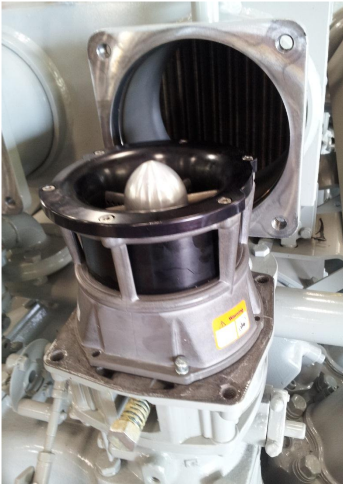
Figure 8: Properly seated venturi assembly.
