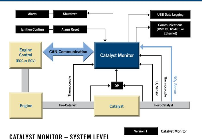
Increased differential pressure across the catalyst indicates masking/fouling of the catalyst elements. A substantial decrease in this differential pressure can indicate severe damage. Our Cat Monitor will log the differential pressure, notify the user of any unacceptable conditions and ensure your engine remains in compliance continuously.
