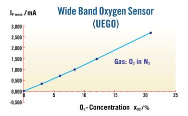
around a more suitable sensor for controlling the AFR of Natural Gas Engines. For this reason, all of CCC's products are designed to accept an input from the Wide Band (UEGO) sensor not the older narrow band sensor. The use of the Wide Band Sensor also allows CCC's AFR products to be used in rich burn applications with less that .5%  $O_2$  in the exhaust to lean burn applications with as much as  $12\% O_2$  in the exhaust.
