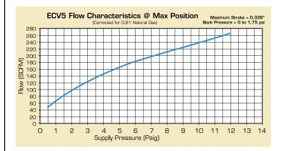
As can be seen from the chart, if the injection pressure is zero and the gas flow is 60 scfm, 1 psi of of gas pressure is required.
