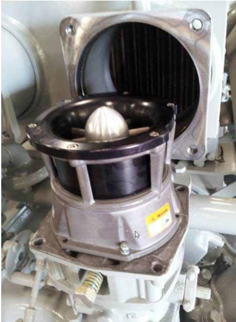
Figure 8: Properly seated venturi assembly.
