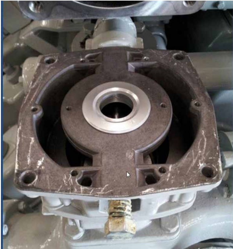
Figure 1: Air horn and air-gas valve assembly have been removed.
