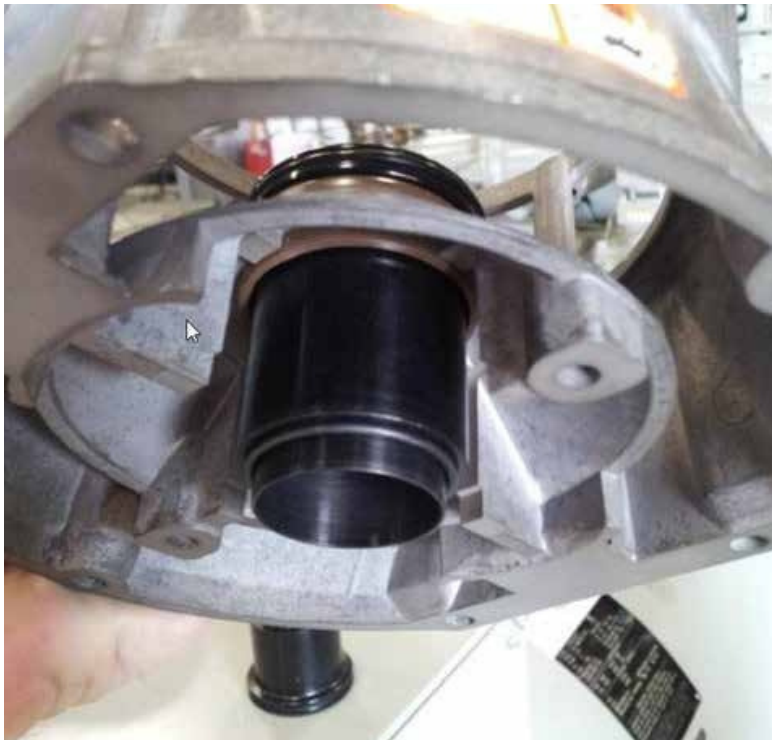
Figure 5: Properly inserted center section
