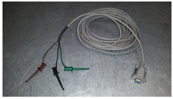
2. Attach the three wire grabbers (Green, Brown, and Black) to the appropriate communication wires on the GV1 Cable.
