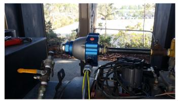
Note: In picture above the carburetor inlet pipe size is  $\frac{3}{4}$ " NPT. The GV1 Inlet and Outlet port is  $1\frac{1}{2}$ " NPT, so bushings were utilized for proper installation.
