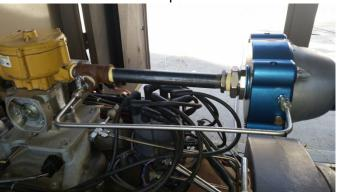
In this illustration the GV1 was mounted approximately 14 "away from the Carburetor. This placement was due to the position of the Distributor.
