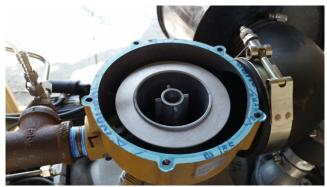
6. Install Venturi assembly into Carburetor.
