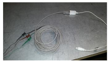
NOTE: PRIOR TO CONNECTING THE USB TO SERIAL PORT ADAPTER CABLE, THE DRIVERS FOR THIS DEVICE WILL HAVE TO BE LOADED TO YOUR LAPTOP AND THE USB TO SERIAL ADAPTER WILL THEN NEED TO BE CONFIGURED TO YOUR LAPTOP. ENSURE THE USB TO SERIAL ADAPTER CABLE IS SET UP TO USE COM 1 ON YOUR LAPTOP. PLEASE SEE YOUR COMPUTER ADMINISTRATOR FOR ASSISTANCE.
