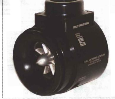
Continental Controls' Mixing Venturi VM-350. The venturi is available in three sizes with variations within each size to accommodate a range of engine sizes. The size and number of fuel injection ports are adjusted for each engine type as necessary. The dimensions of the VM-350, sized for 350 hp engine with stoichiometric air/fuel ratio are 5 in. (12.7 cm) length, 6 in. (15.2 cm) diameter, flanges as required.
