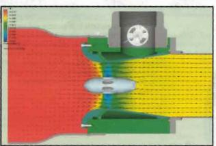
Crossection view of Continental Controls' air/fuel mixing venturi. The air inlet of the venturi is on the left. The dark green area is the measurement of throat pressure and is a result of the airflow through the venturi as sensed by the holes around the throat area. The gas inlet is on the top of the venturi. Gas is injected through multiple holes located around the periphery of the throat and the many holes
