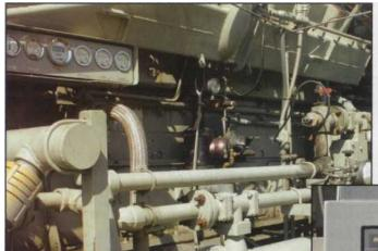
■ The engine uses a Continental Controls Corporation ECV 5 valve seen here in the center of the photo, and a computerized monitoring and display unit (inset photo) to control fuel delivery and pressure.
