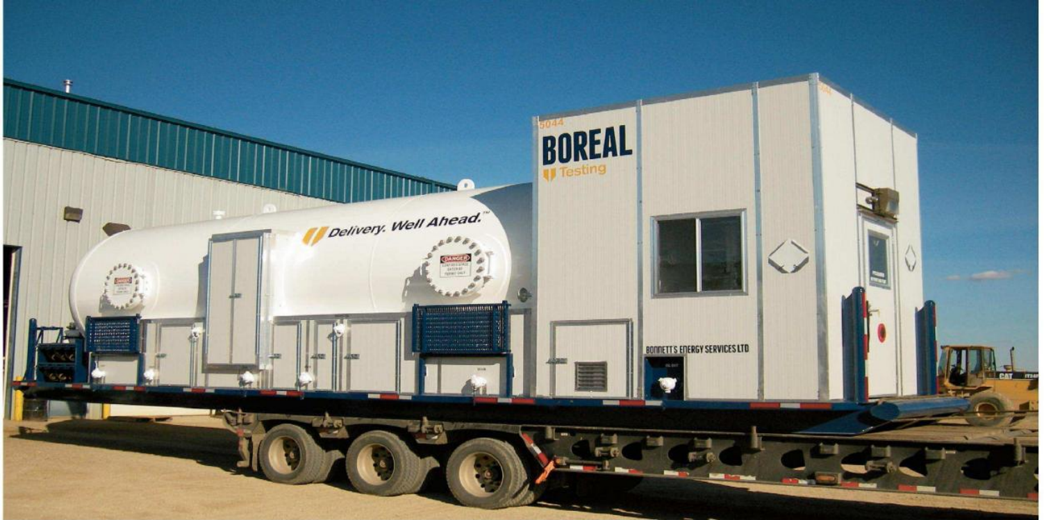
Production Testing Skid With Skirted Vessel At Operator's Control Building
