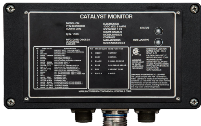
The CCC Cat Monitor is available as a Data Logger and a real-time emissions controller with a CCC AFR valve system.
